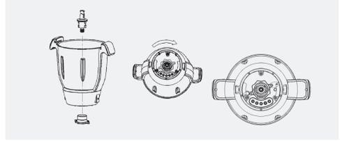
Place the drive shaft correctly locked into the jug.
