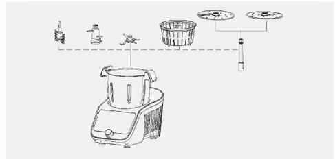
Choose difference accessories for difference cooking purpose. **Note: The whisk should be used with the blade.**
