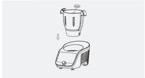
Insert the Jug into the Main Unit. Press down firmly to lock into place. (LOGO in front), Max in back).
